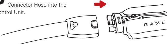
To disconnect, simply press the blue or gray button and remove the connector from the Wrap.
